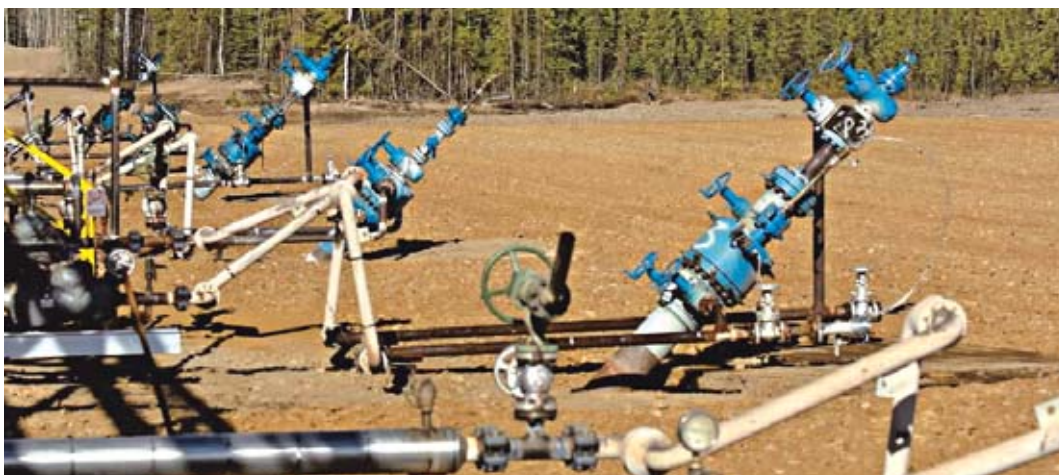
Wellheads at the Joslyn site, in the Athabasca area (Province of Alberta, Canada), used by the Total Group for the extraction of tar sands (containing extra-heavy crude oil) by steam-assisted gravity drainage (SAGD process).
