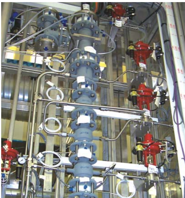
Charged with iodine in November 2006, the Bunsen reactor, for the investigation of the iodine-sulfur thermochemical cycle, constructed by CEA, and photographed at Marcoule before being sent to the United States, where it is to be coupled to the other two components of a complete pilot plant, under the aegis of a CEA-DOE agreement. The dissociation installations for sulfuric acid, and hydriodic acid are constructed, respectively, by Sandia National Laboratories, and General Atomics.
